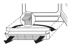
With the door closed, remove the cross-head screws from the lower door bearing and remove the door bearing downwards.
